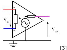
$V_{out} = A V_{in} = A (V^+ - V^-)$  where A is the open-loop gain of the op-amp. [2]
