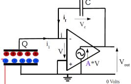
Using an integrating circuit,  $V_{\mbox{\scriptsize out}}$  is proportional to charge and hence proportional to acceleration.
